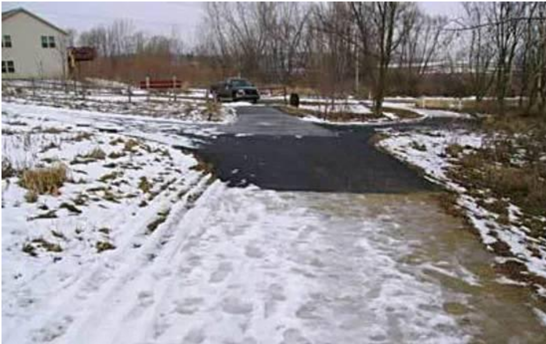
A test section shows how well snow has melted on the porous asphalt Section (center) compared to the crushed rock trail (foreground) and regular asphalt (far left and rear)
