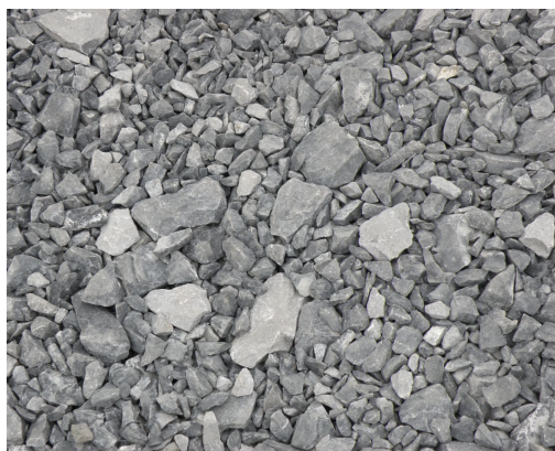
Figure 2. Bigger Aggregates of Asphalt for Choker Layer (2013) From AsphaltPro
