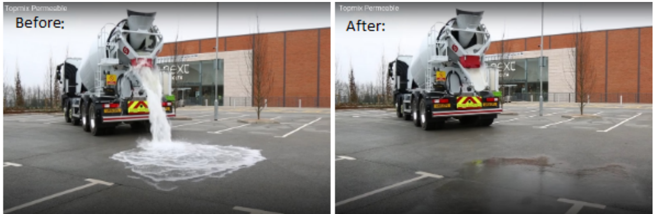
Figure 2. Topmix permeable before and after shot (2019). From Topmix Permeable - Designing Buildings.
