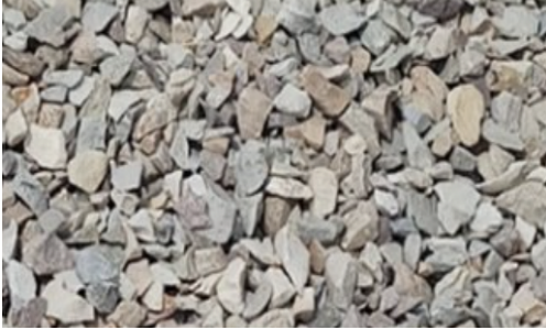
Figure 3. Crushed Stone for Sub-Base Reservoir (2020) From Ahmed, Tanveer
